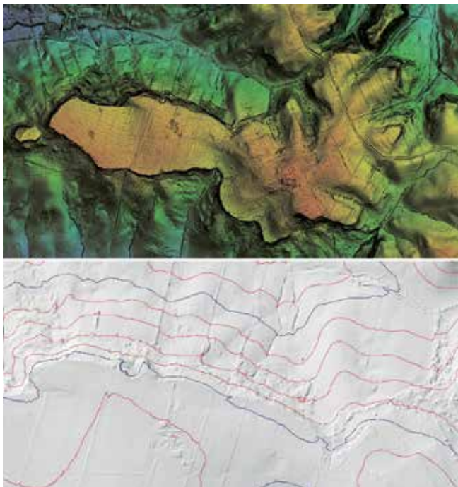
Figure 3. Contour lines every 0.25 meter on DTM without vegetation and contour lines every meter on the 3D model
