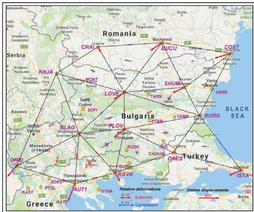
Figure 3. Relative side and principal deformations and vectors of station displacements for the time span 2011-2016. Relative deformations of 5 \cdot 10^{-7} correspond to 5mm compression (in blue) or extension (in red) per 10km.
