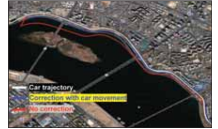
Fig.15 Position error in turning
