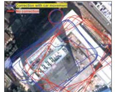
Fig.18 Estimated position in underground parking
