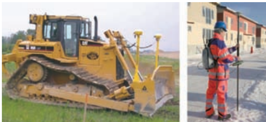
Figure 4: Two increasingly common production applications for SWEPOS positioning services are machine guidance and detail surveying (e.g. for mapping purposes)
