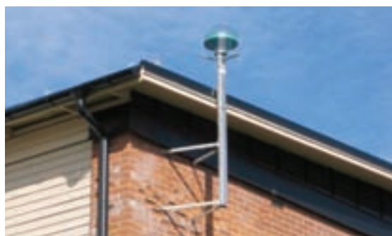
Figure 3: A SWEPOS station with a roof-mounted antenna, belonging to Class B.
