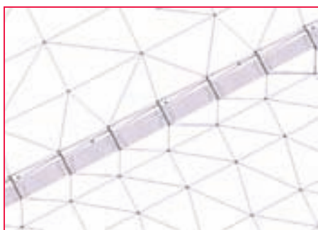
Figure 5: TIN interpolation on the points leaning towards a building (top view)
