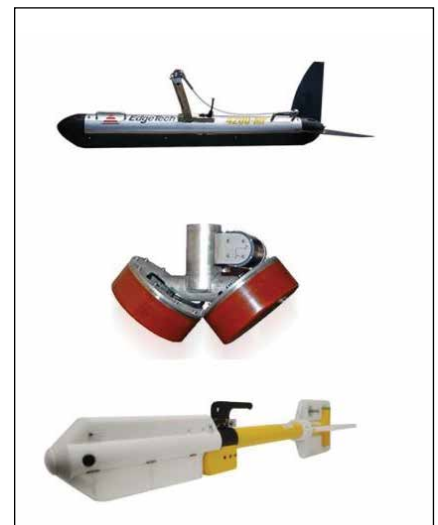
Figure 1. Survey equipment used (from top to bottom order): Edgetech sidescan sonar Edgetech 4200, Multibeam echosounder Kongsberg EM3002 dual head, Magnetometer Geometrics G-882
