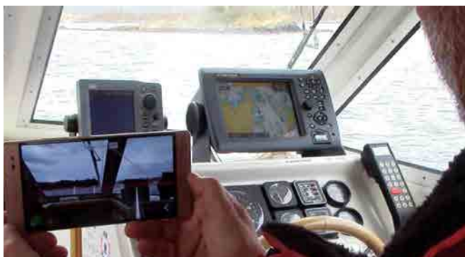
Figure 4. The test application on the smartphone (Lenovo Phab 2 Pro) during the pilot test. To the right the boats reference stationary chart plotter
