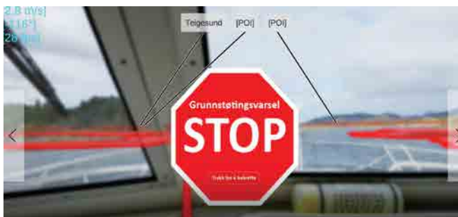
Fig. 6. Screen dump from the Galaxy test phone. The grounding alarm has been triggered with both an aural and a visible alarm
