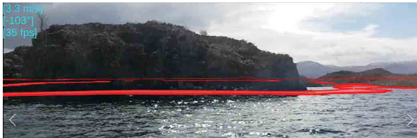
Fig. 7. The picture show the offset of the AR layer with the red NoGo areas as they were fluctuating due to noise in the phones internal compass. However, users judged in acceptable during the tests
