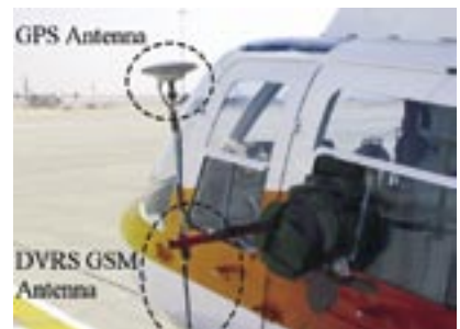
Figure 2. System installation for the helicopter test
