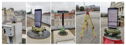
Figure 1. Smartphone und reference receiver SP80 on two neighbouring measuring pillars on the roof of the El building of TU Wien and mobile measuring set-up on Karlsplatz.
