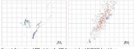
Figure 4. Comparison of PPP solutions for GPS (turquoise) and GLONASS (purple); on the left is point N09, on the right N07. Solutions for which only one SPP solution could be determined are shown in red. Note, the different scale of the grids.
