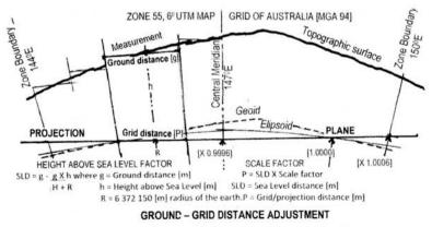
Ground distance [g] dimension is the distance on the horizontal plane at the mean elevation of its measurement Grid [or Projection] distance [P] is the distance on the Projection Plane and is Ground distance adjusted for Height above Sea Level and for the Scale Factor of the co-ordinate projection.
