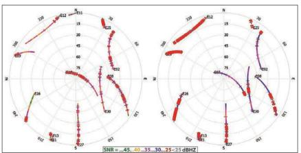
Figure 3. Skyplots showing the tracked Galileo satellites of the Google Pixel 5 on E1 (left) and E5a (right) with coloured visualisation of the Signal to Noise Ration (SNR).
